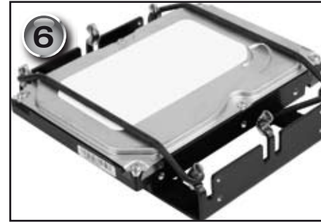
8. Slide the outer string of the second rubber band over the HDD and center the drive between the rubber bands (fig. 6).
