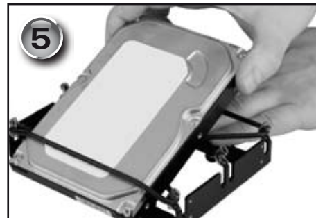
7. Pull up the outer string of a rubber band and carefully slide the HDD into the gap (the strings of the rubber bands which are tied together by the cable tie go underneath the HDD) (fig. 5).
